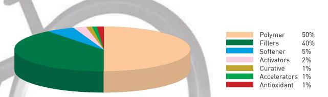
All additives affect the properties of the rubber material. A rubber material developed for a certain product is seldom useful in other applications. For technically more advanced products there are always specially developed materials to fulfill the specific demand.
